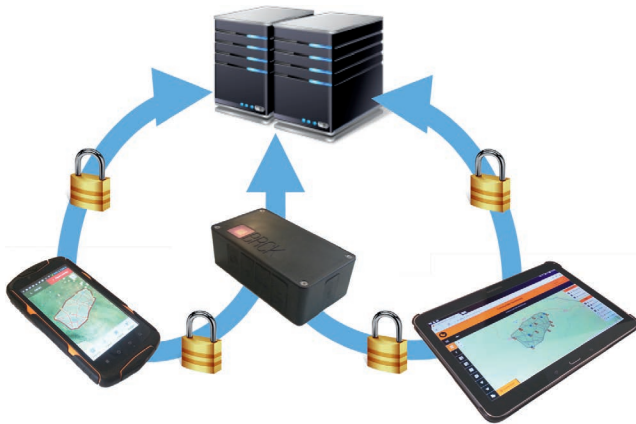
Figure 9 The C3 system exchanges information through a cloud based database, and the ranger device communicates with the cloud either directly over the cellular network, or via a wifi hotspot (BRCK) at their stations, which in turn is connected to the cellular network with external antennas and amplifiers. All data are encrypted and access relies on state of the art authentication procedures.
